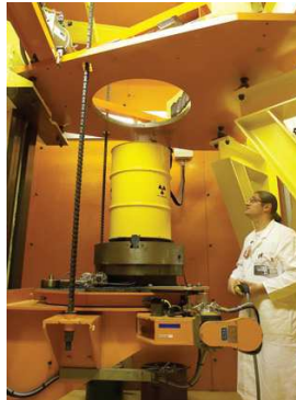
TRANSEC station capable of accommodating irradiating packages up to 200 litres / 500 kg
