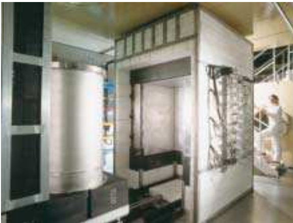
SYMETRIC neutron measurement cell designed to characterise fissile material in irradiating packages
