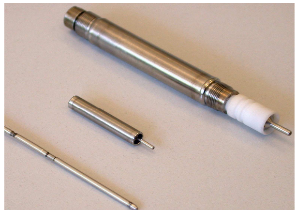
Fission chambers (Ø1.5 mm, 4 mm, 8 mm)
